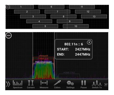
To enable the Wi-Fi channel guide, tap located in the top left corner. Then, tap any of the boxes listed (1-13) to highlight channel activity. To hide the Wi-Fi guide, just tap
