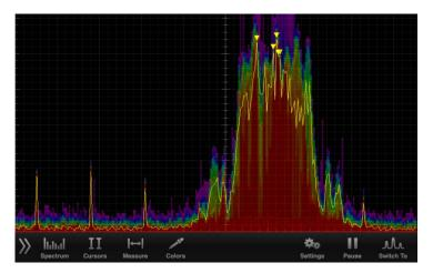
**Raw** – represents the raw spectral data and is visualized by the blue squiggly line. The problem with raw view is the signals are so fast that it's impossible to do anything with the data. Image captures here:
