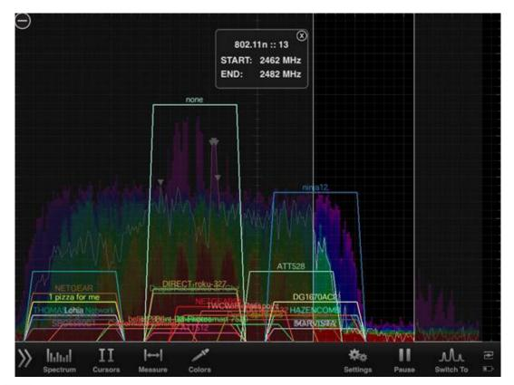
In this example, there is no clear channel in 2.4 GHz. This interference was limited to the inside of the home (interference was not visible when leaving the residence). In this example although 2.4 GHz was very congested, 5 GHz was not. It was recommended that the customer add dual band adapters on wireless devices to utilize 5 GHz for best speeds...or accept slower speeds on 2.4 GHz.
