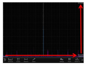
The arrow pointing up represents amplitude. The higher the signals are on the screen, the stronger the signal.
