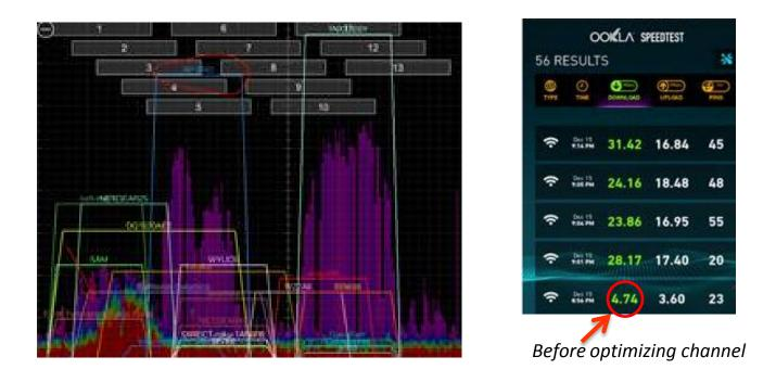
Best practices include using channels 1, 6 and 11 only for deployment of Wi-Fi over 2.4 GHz since these channels represent non-overlapping frequencies. Channels on 5 GHz do not overlap. The example above is for illustration purposes only, that manually selecting channels does impact wireless speed.
