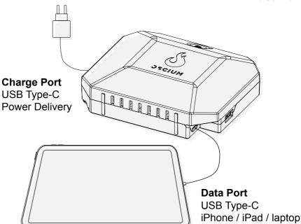
Nomad comes equipped with a fast charge PD power supply. For shipments to customers in the US, a Type A connector will be included. For customers in Europe, a Type C connector will be included.
